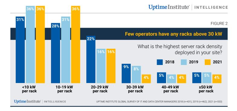
When we asked owners and operators about their highest density racks — and exclude high performance compute (HPC) operations — few (one in 10) have any above 30 kW. About one in six have maximum densities of 20-30 kW racks.
